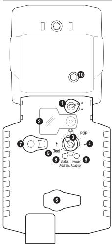
Direction of stroke switch Switch over: Direction of stroke changes
